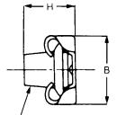
UPPER THREADED PORTION DEFORMED ELLIPTICALLY TO PRODUCE SELF-LOCKING ACTION
